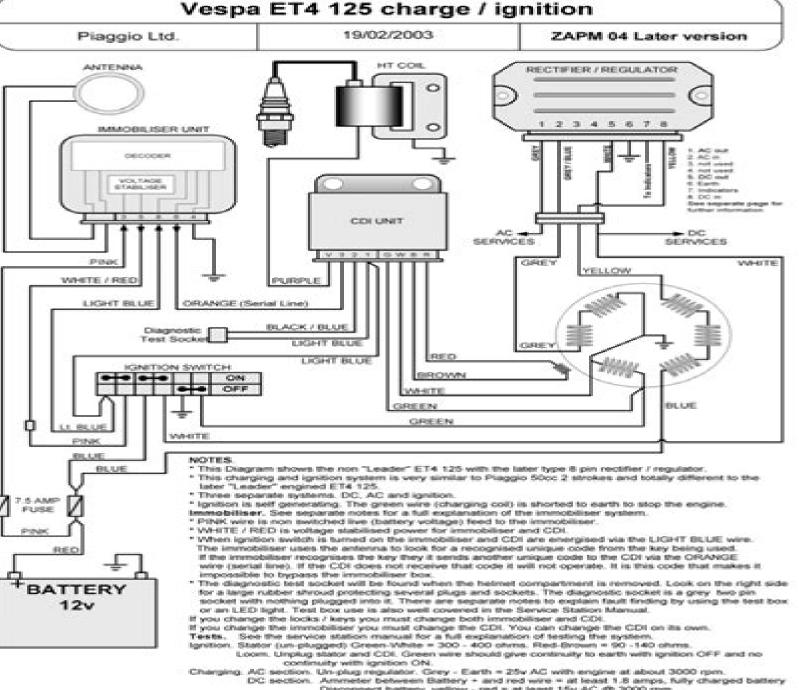
Disconnect battery, yellow - red = at least 15v AC @ 3000 rpm.
