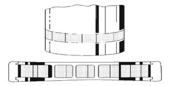
Fig. 4: Identifying Brinelling Courtesy of GENERAL MOTORS CORP.
